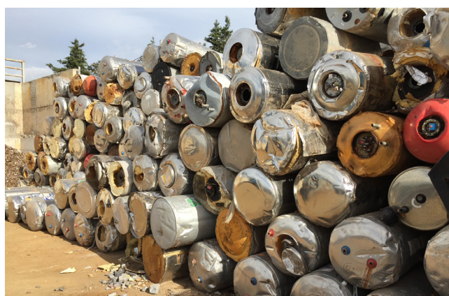
Figure 4: Boilers for manual PU foam removal and processing in refrigerator recycling plants (picture used with the kind permission of the RAL Quality Assurance Association for the Demanufacture of Refrigeration Equipment, 2020).
