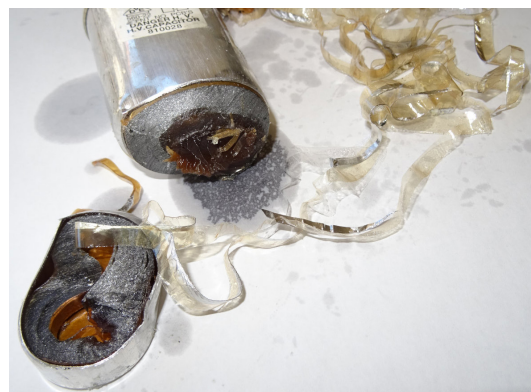
As the dismantling shows, the microwave capacitor is heavily impregnated
