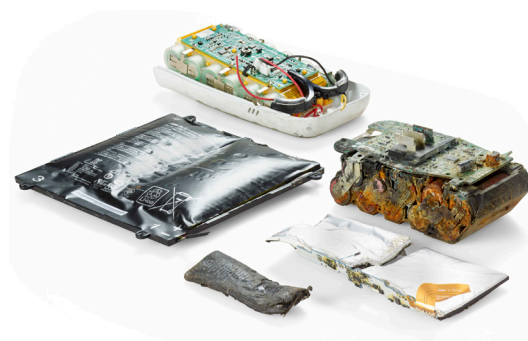
The risk of fire is increased particularly if LiBs are defective. (Photo: INOBAT)
