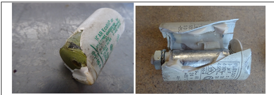
Figure 21: Opened plastic capacitors without liquid substances
